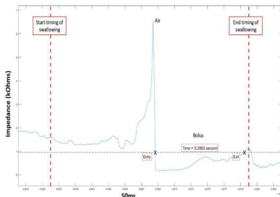
**Figure 3:** Impedance change measured during the bolus transmit over a single impedance channel. A rapid increase in the impedance channel is noted when the air through the impedance segment. The drop in the impedance channel is the higher conductive bolus material passes through the measuring site. The criteria is fulfilled the bolus successfully transmit through the region which the impedance located in the transition zone of esophagus.
